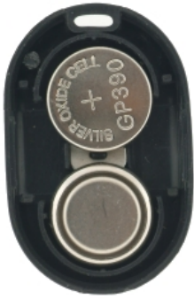
Figure 4: Replacing the Home Tag Battery
