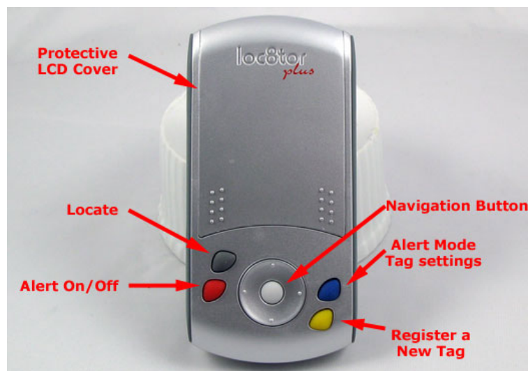
Figure 10: Controls Layout on the Loc8tor
